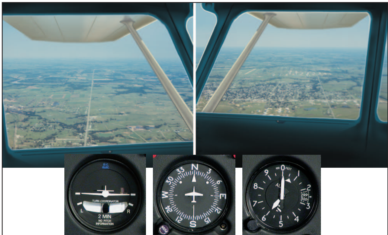
Figure 3-4. Wingtip reference for straight-and-level flight.
