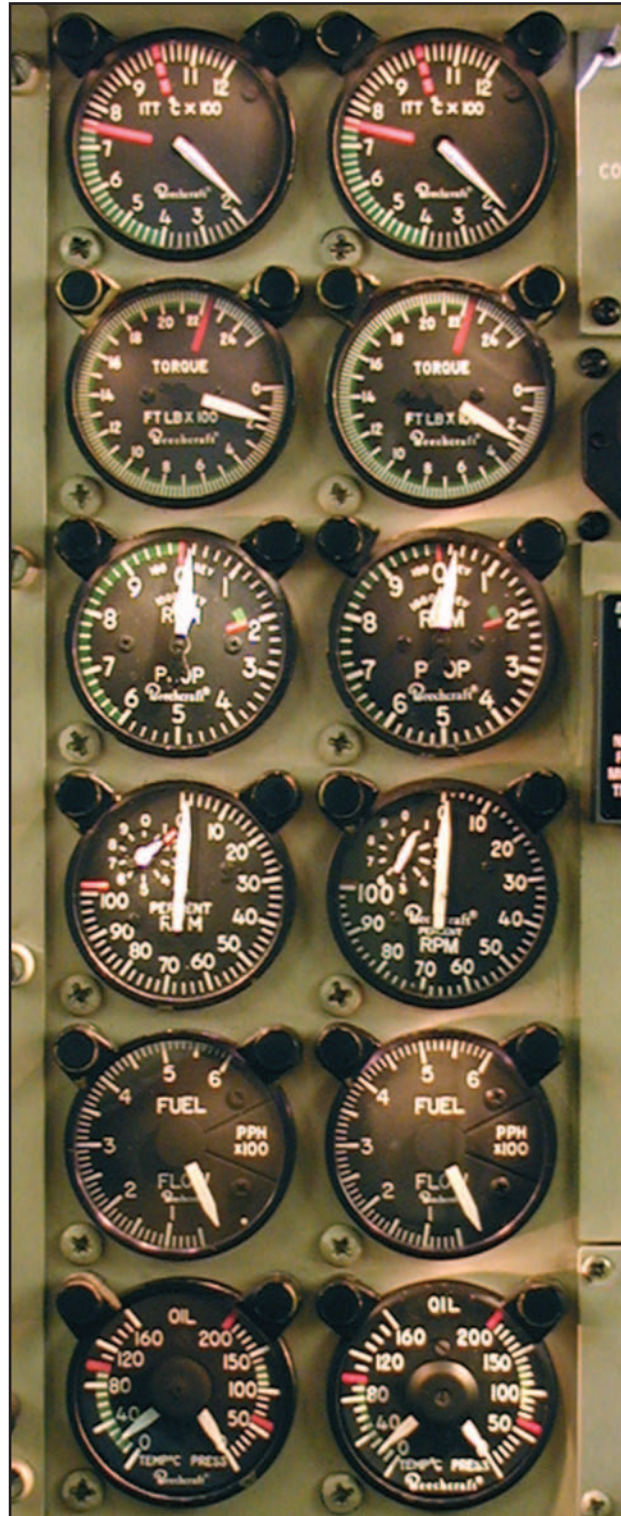
Figure 14-7. Engine instruments—split shaft/free turbine engine.
