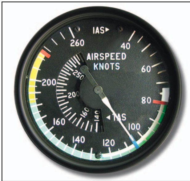
Figure 12-1. Airspeed indicator markings for a multiengine airplane.
