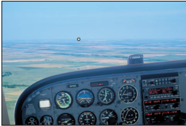
Figure 3-11. Visual reference for angle of bank.
