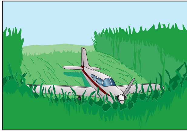
Figure 16-1. Using vegetation to absorb energy.
