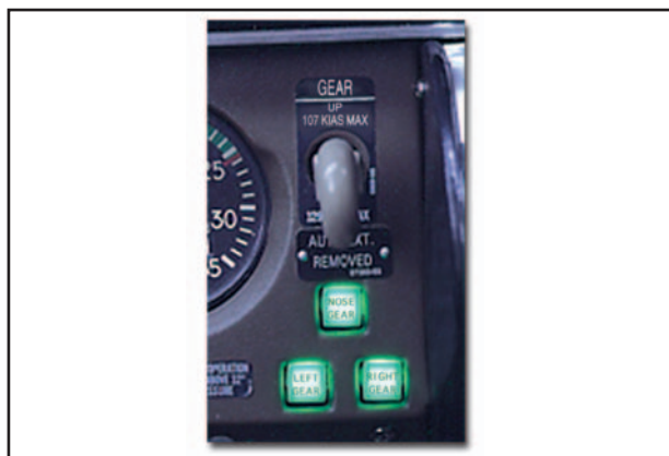
Figure 11-6. Typical landing gear switches and position indicators.
