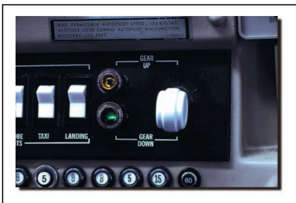
Figure 11-7. Typical landing gear switches and position indicators.
