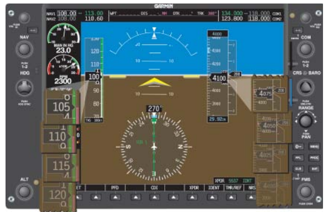
Figure 5-55. An aircraft decreasing in airspeed while gaining altitude. In this case, the pilot has decreased pitch.
