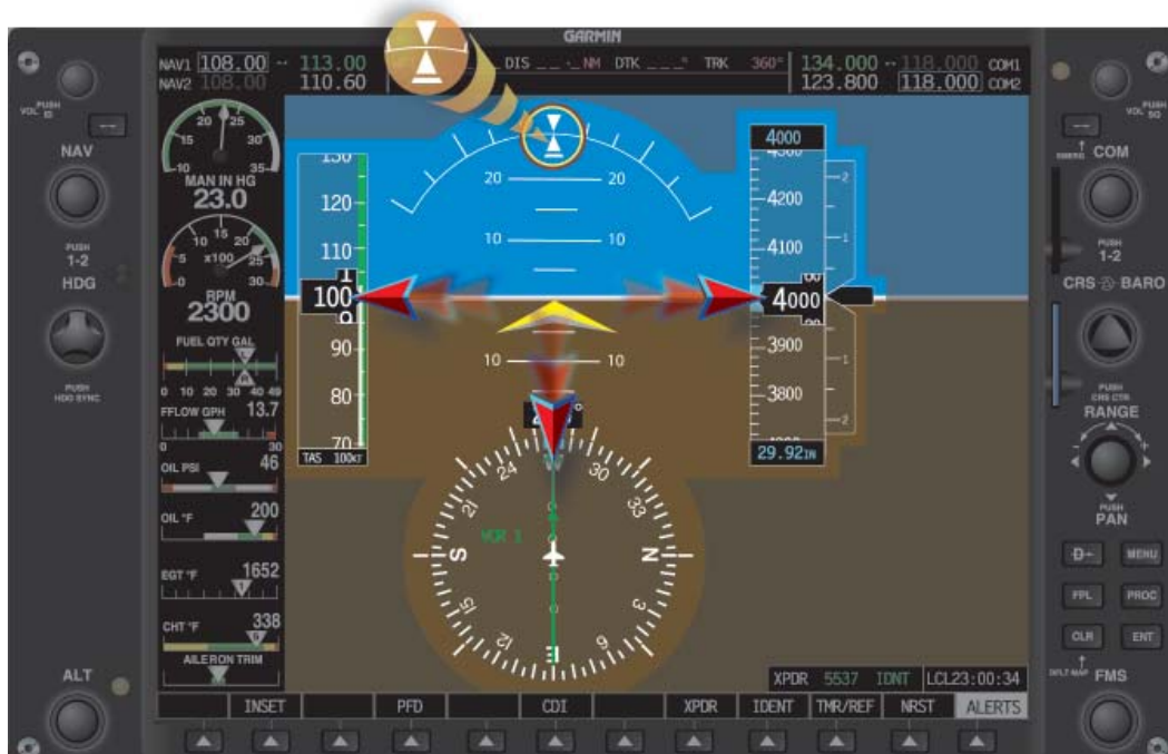
Figure 4-34. Selected Radial Cross-Check.
