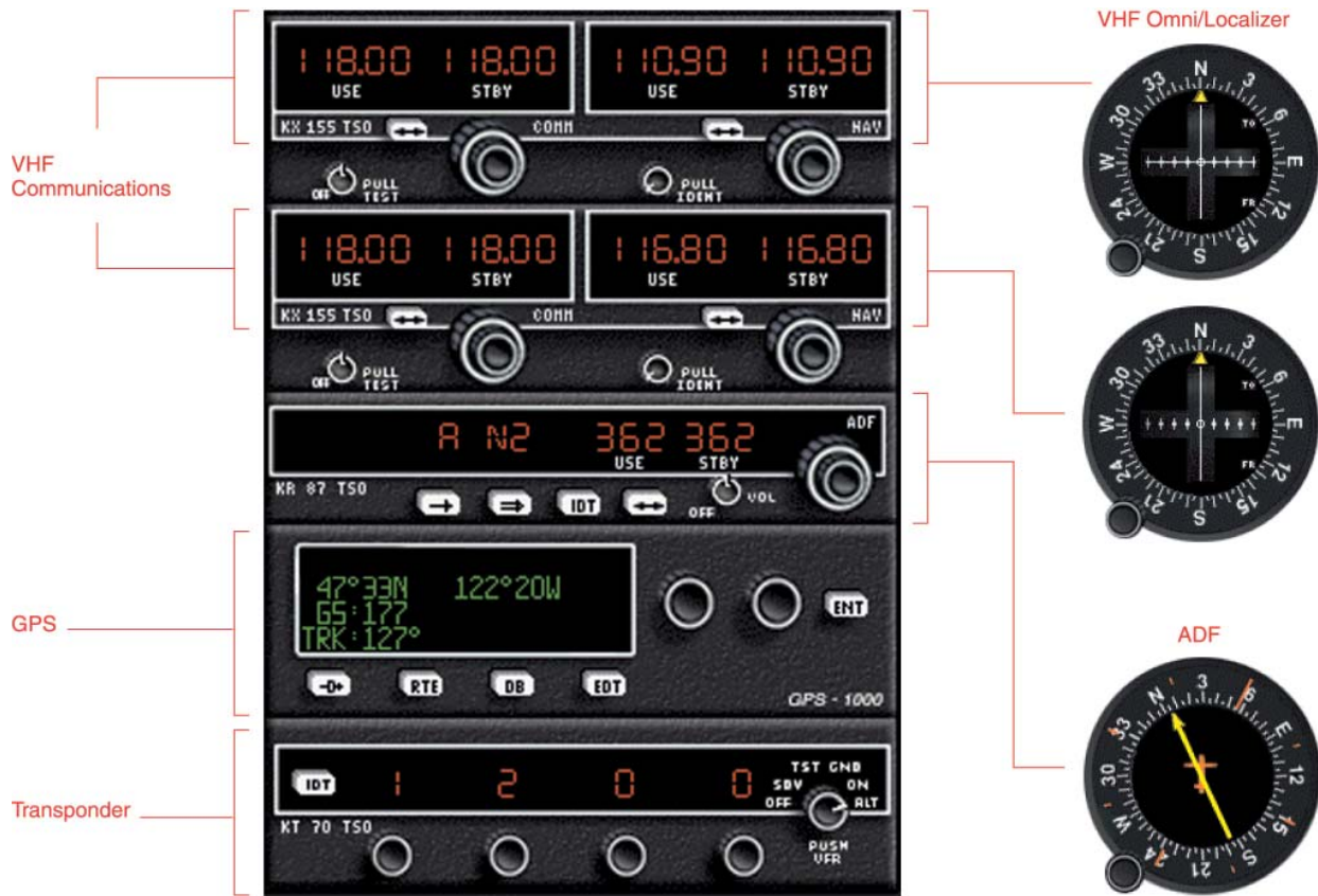
Figure 9-1. Typical NAV/COM Installation.
