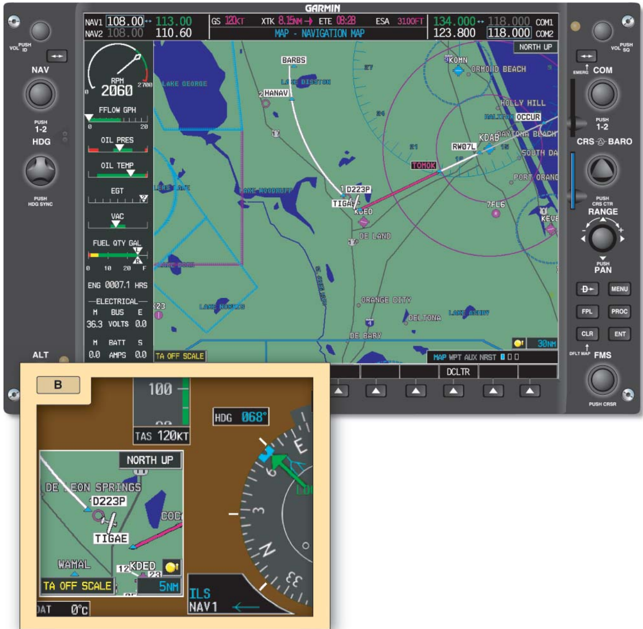
Figure 7-20. The same aircraft illustrated in Figure 7-19 shown on the ORM radial near TIGAE intersection turning inbound for the localizer.
