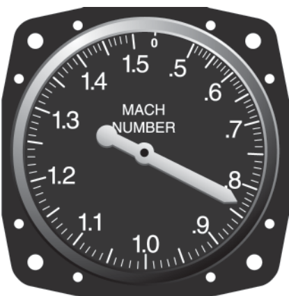
Figure 3-13. A Machmeter shows the ratio of the speed of sound to the TAS the aircraft is flying.
