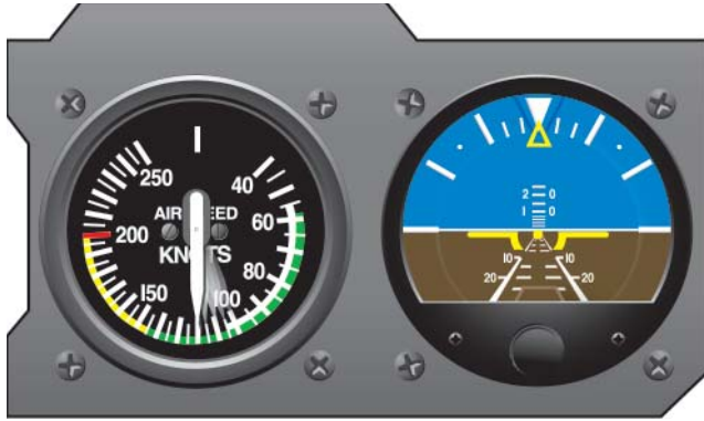
Figure 4-9. Pitch attitude has lowered.
