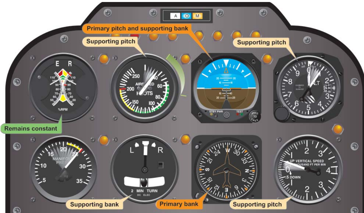
Figure 6-16. Flight Instrument Indications During an Instrument Takeoff.
