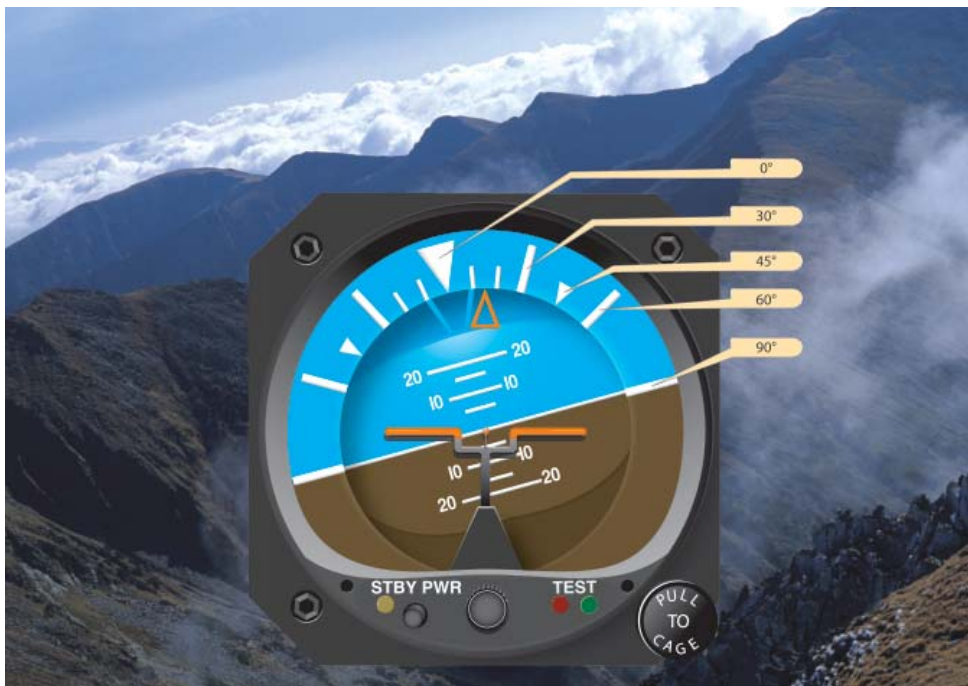
Figure 6-5. The banking scale at the top of the attitude indicator indicates varying degrees of bank. In this example, the helicopter is banked approximately 15° to the right.
