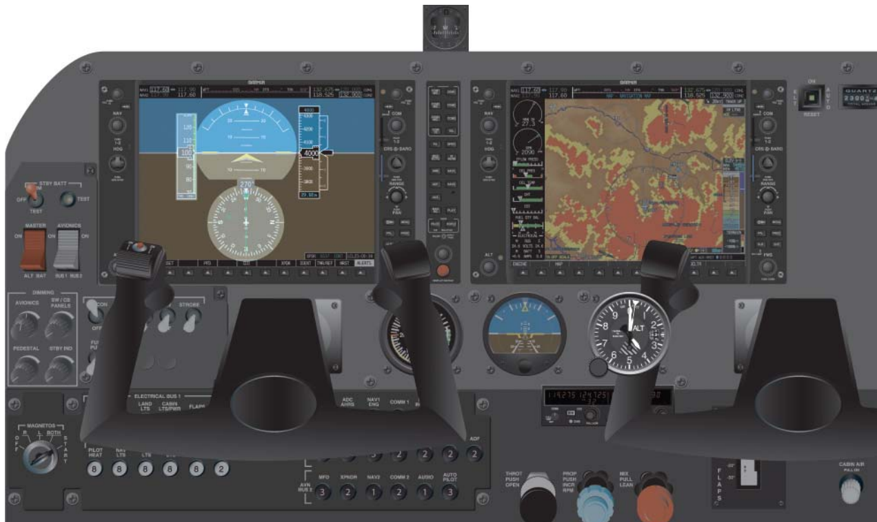
Figure 4-33. Note that the altitude and vertical speed tapes are slightly to the right of the pilot’s direct forward line of sight.
