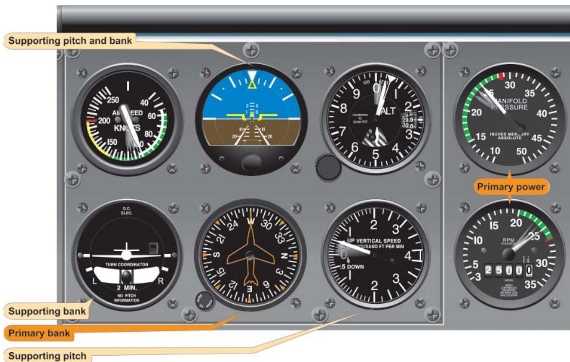
Figure 5-25. Climb Entry for Constant Airspeed Climb.
