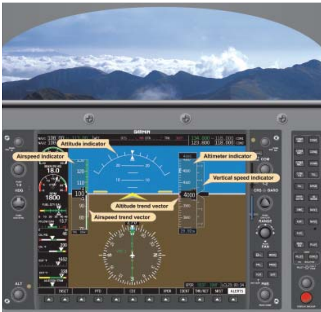
Figure 5-47. Pitch Attitude and Airspeed in Level Flight, Slow Cruise Speed.
