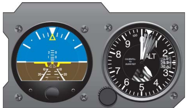
Figure 4-7. Pitch Correction Using the Altimeter.
