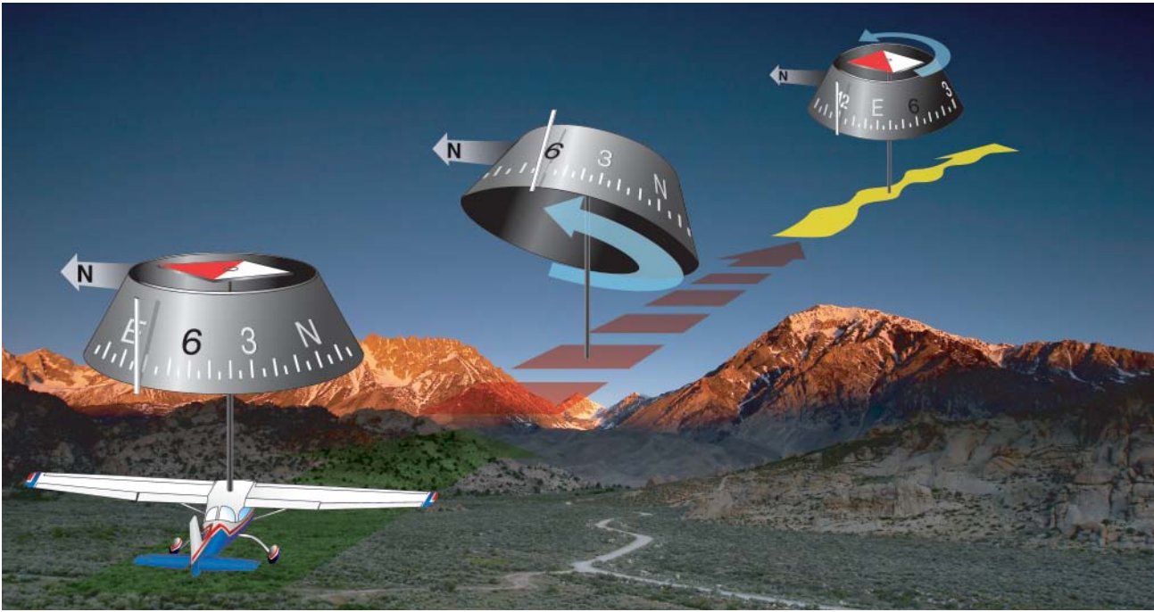
Figure 3-21. The Effects of Acceleration Error.
