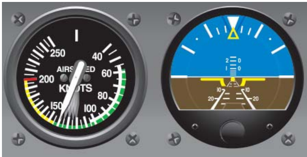
Figure 5-14. Constant Power Plus Decreased Pitch Equals Increased Airspeed.
