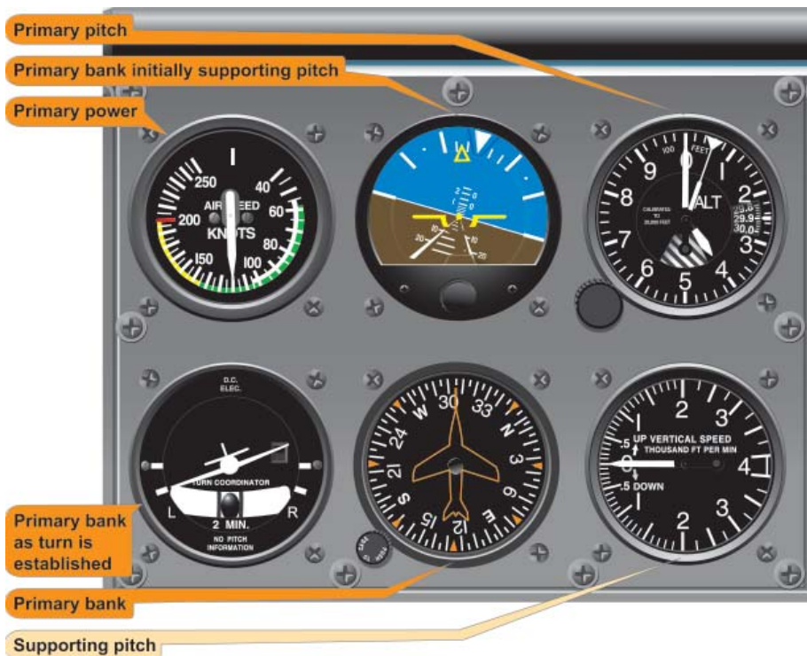
Figure 5-33. Standard Rate Turn, Constant Airspeed.
