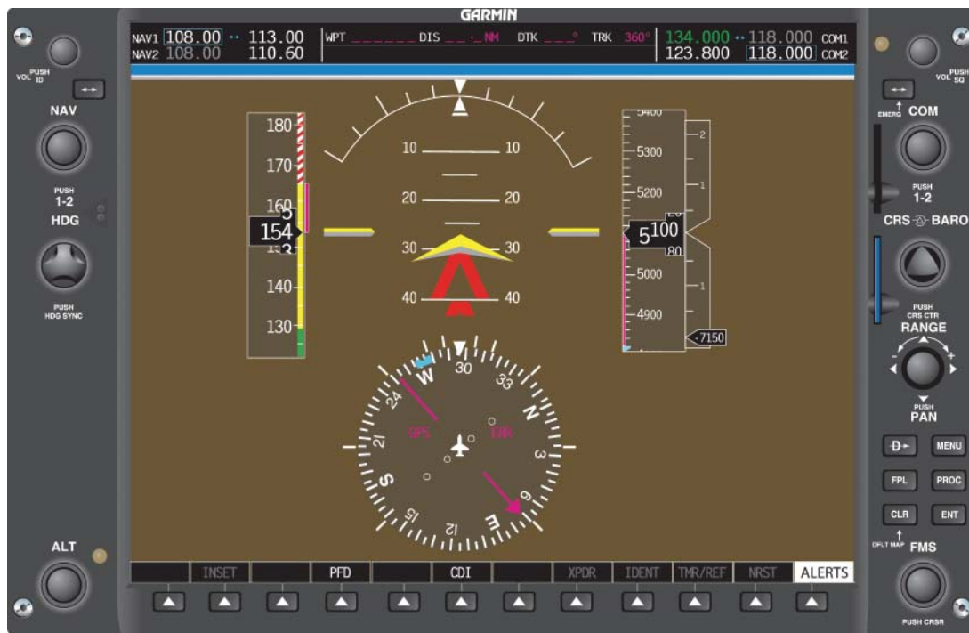
Figure 5-70. Horizon line starts moving upward at 27°. Note that the blue sky remains visible at 17° nose-down.
