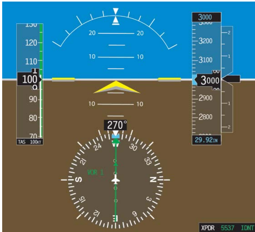
Figure 6-17. PFD Indications During Straight-and-Level Flight.
