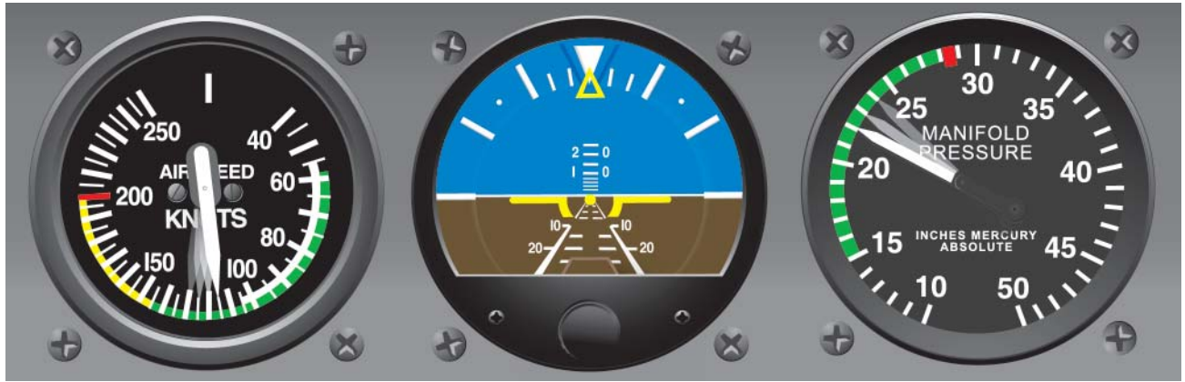
Figure 4-14. Pitch Control and Power Adjustment Required To Bring Aircraft to Level Flight.
