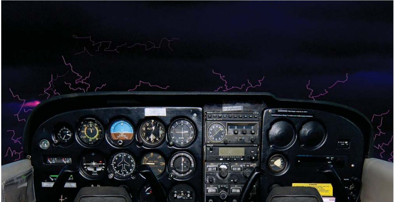
Figure 11-1. St. Elmo's Fire is harmless but may affect both communication and navigation radios, especially the lower frequencies such as those used on the ADF.
