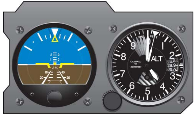
Figure 4-6. Pitch Correction Using the Attitude Indicator.
