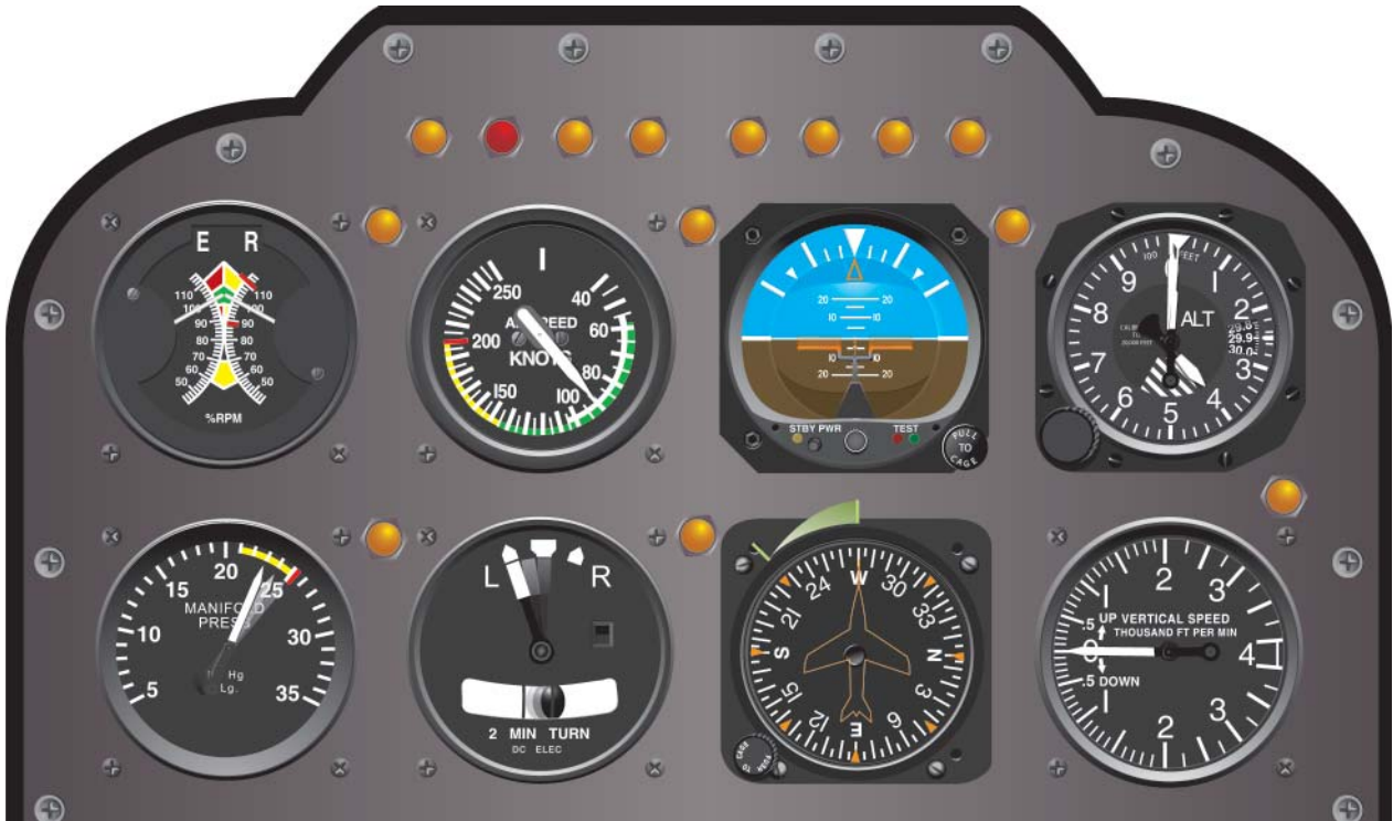
Figure 6-8. Flight instrument indications in straight-and-level flight with power decreasing.
