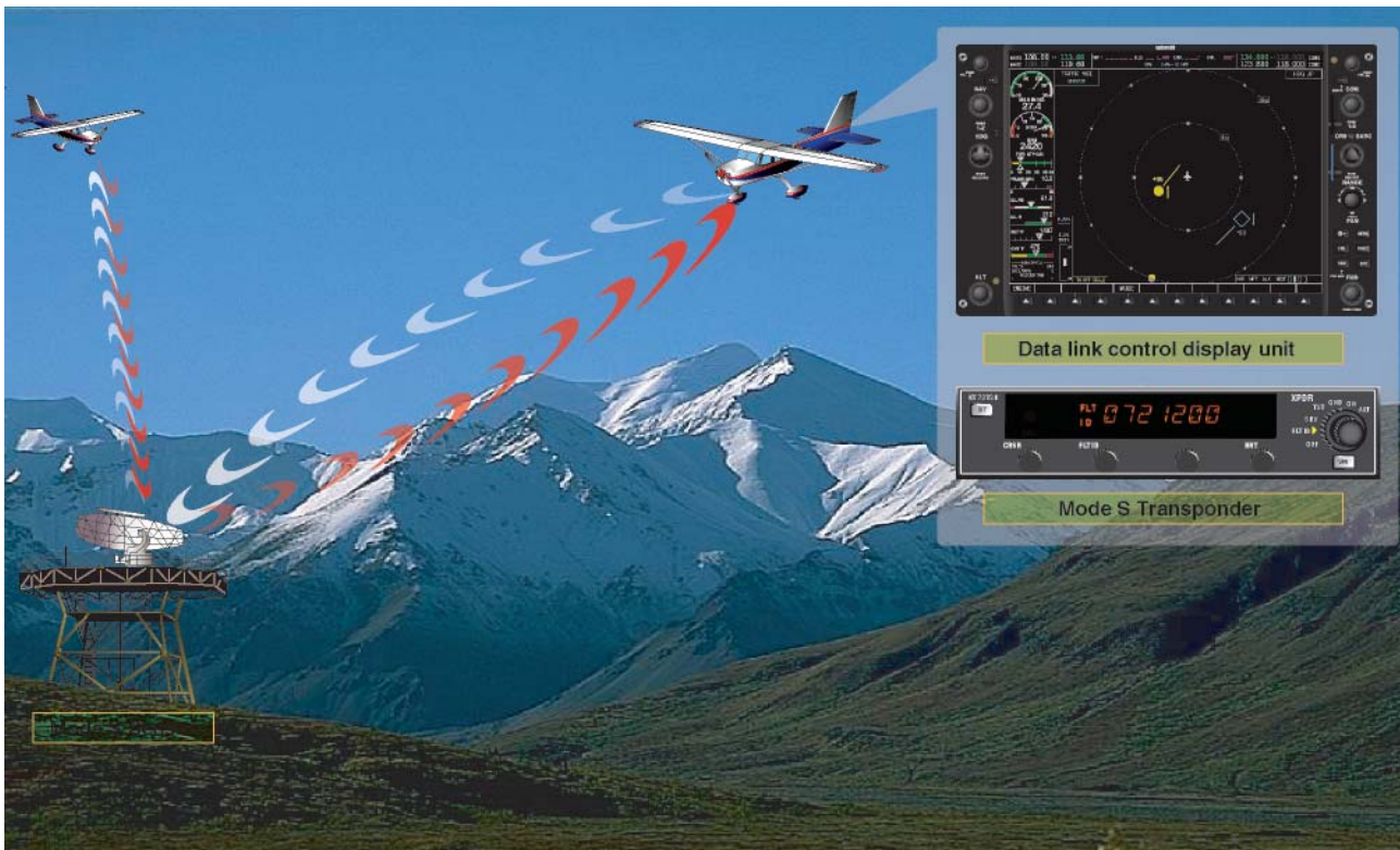
Figure 3-54. Concept of the Traffic Information System.
