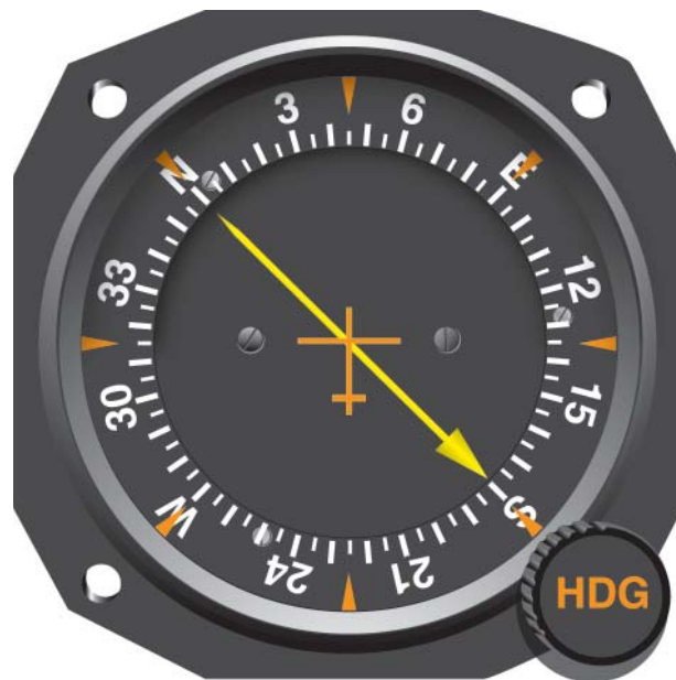
Figure 7-4. Relative bearing (RB) on a movable-card indicator. By placing the aircraft's magnetic heading (MH) of 045° under the top index, the relative bearing (RB) of 135° to the right will also be the magnetic bearing (no wind conditions) which will take you to the transmitting station.
