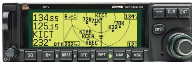
Figure 7-23. Onboard RNAV receivers have changed significantly. Originally, RNAV receivers typically computed combined data from VOR, VORTAC, and/or DME. That is generally not the case now. Today, GPS such as the GNC 300 and the Bendix King KLS 88 LORAN receivers compute waypoints based upon embedded databases and aircraft positional information.
