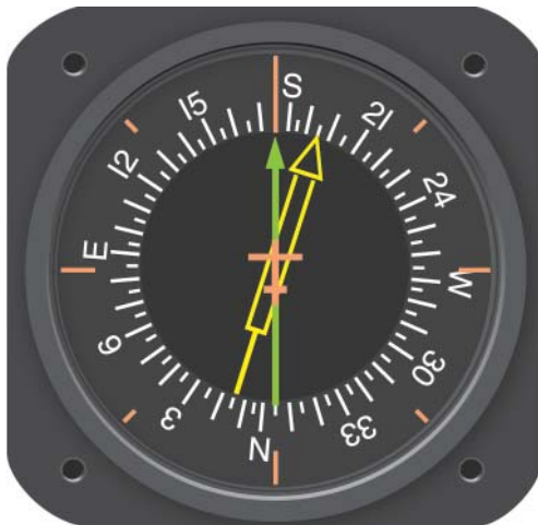
Figure 3-26. Driven by signals from a flux valve, the compass card in this RMI indicates the heading of the aircraft opposite the upper center index mark. The green pointer is driven by the ADF.
