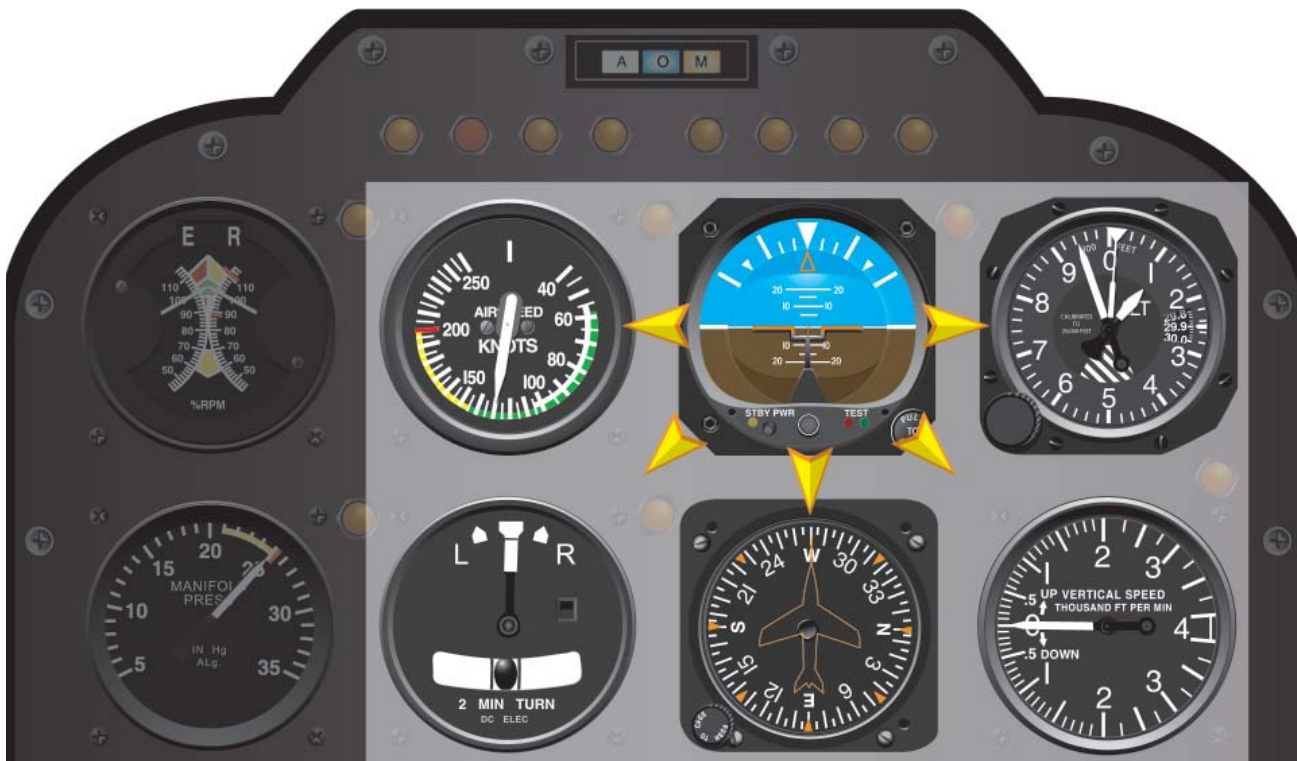
Figure 6-1. In most situations, the cross-check pattern includes the attitude indicator between the cross-check of each of the other instruments. A typical cross-check might progress as follows: attitude indicator, altimeter, attitude indicator, vertical speed indicator, attitude indicator, heading indicator, attitude indicator, and so on.
