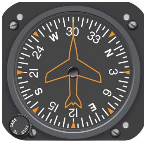
Figure 3-31. The heading indicator is not north seeking, but must be set periodically (about every 15 minutes) to agree with the magnetic compass.
