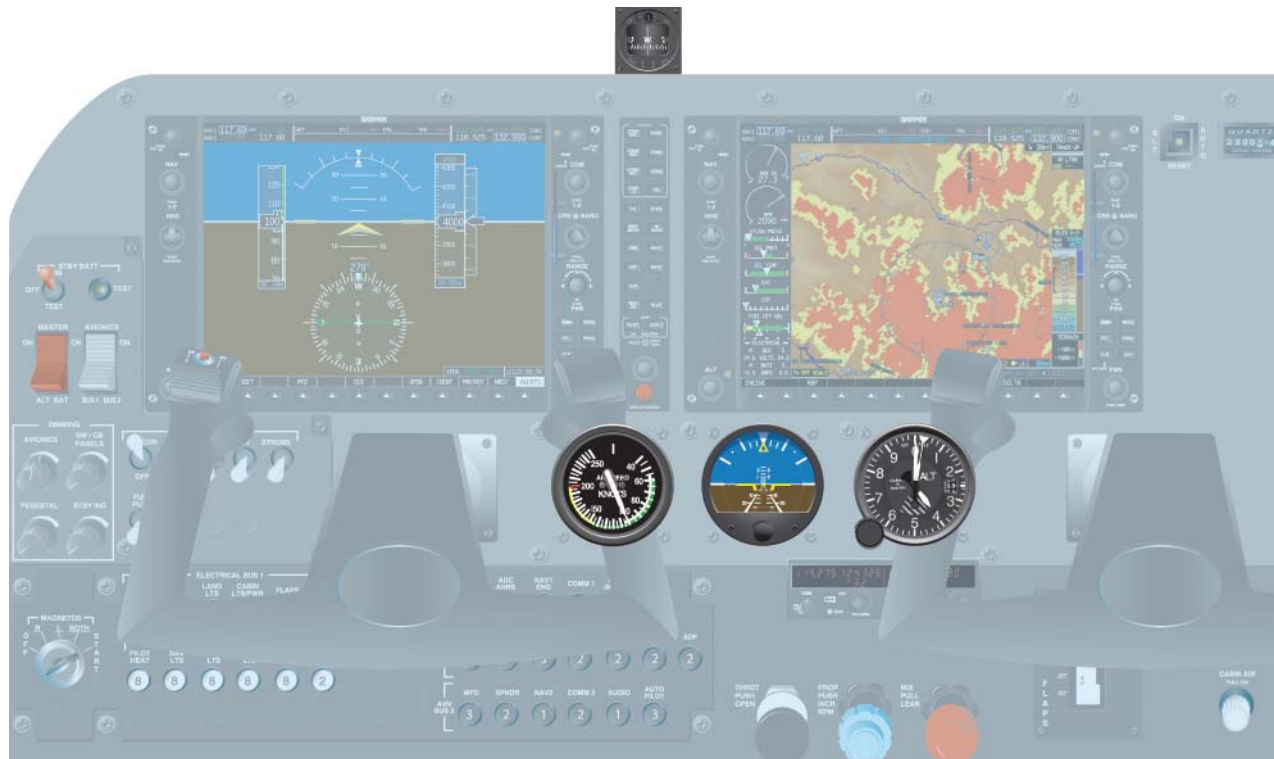
Figure 4-24. Emergency Back-up of the Airspeed Indicator, Attitude Indicator, and Altimeter.
