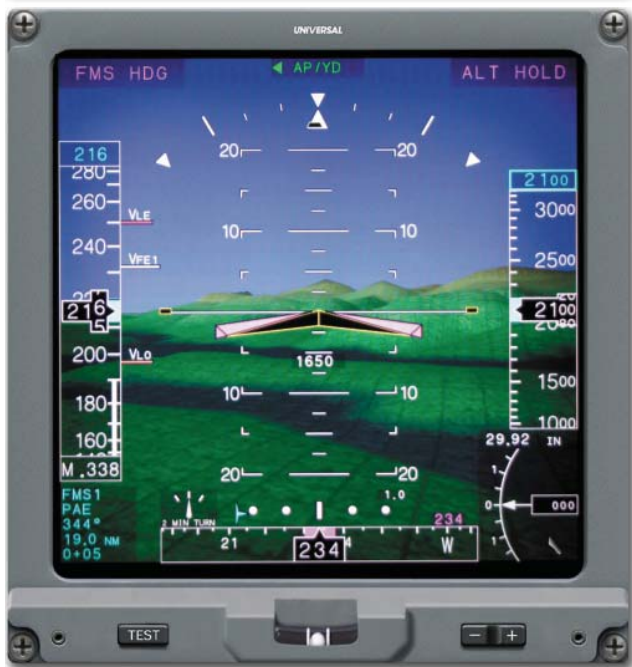
Figure 7-44. Example of a Head-Up Display (top) and a Head-Down Display (bottom). The head-up display presents information in front of the pilot along his/her normal field of view while a head-down display may present information beyond the normal head-up field of view.
