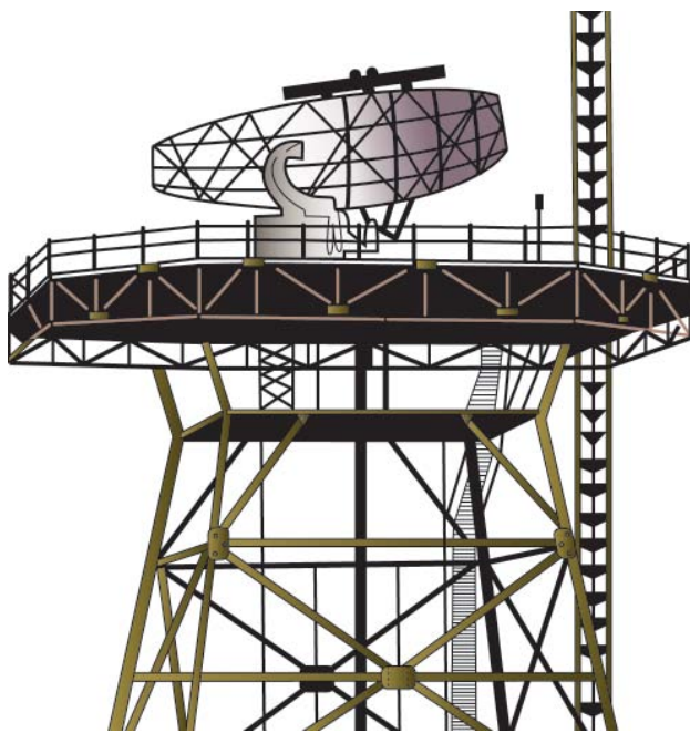
Figure 9-7. Combined Radar and Beacon Antenna.
