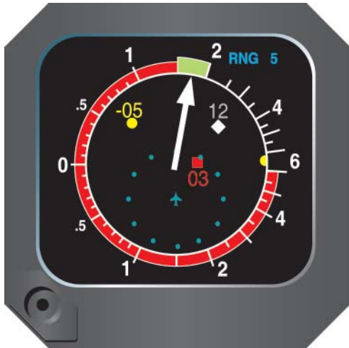
Figure 3-58. An example of a resolution advisory being provided the pilot. In this case, the pilot is requested to climb, with 1,200 feet being the appropriate rate of ascent to avoid traffic conflict. This visual indication plus the aural warning provide the pilot with excellent traffic awareness that augments see and avoid practices.
