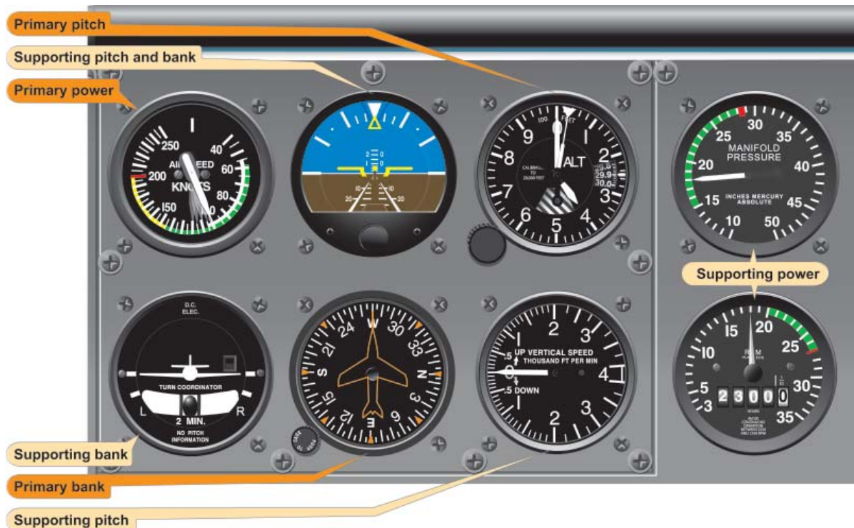
Figure 5-24. Straight-and-Level Flight (Reduced Airspeed Stabilized).
