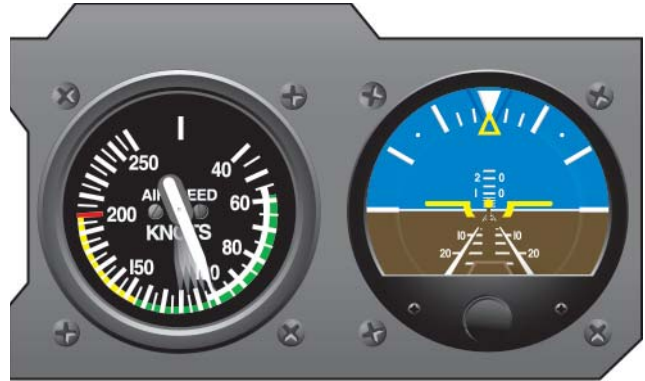
Figure 4-10. Pitch attitude has moved higher.
