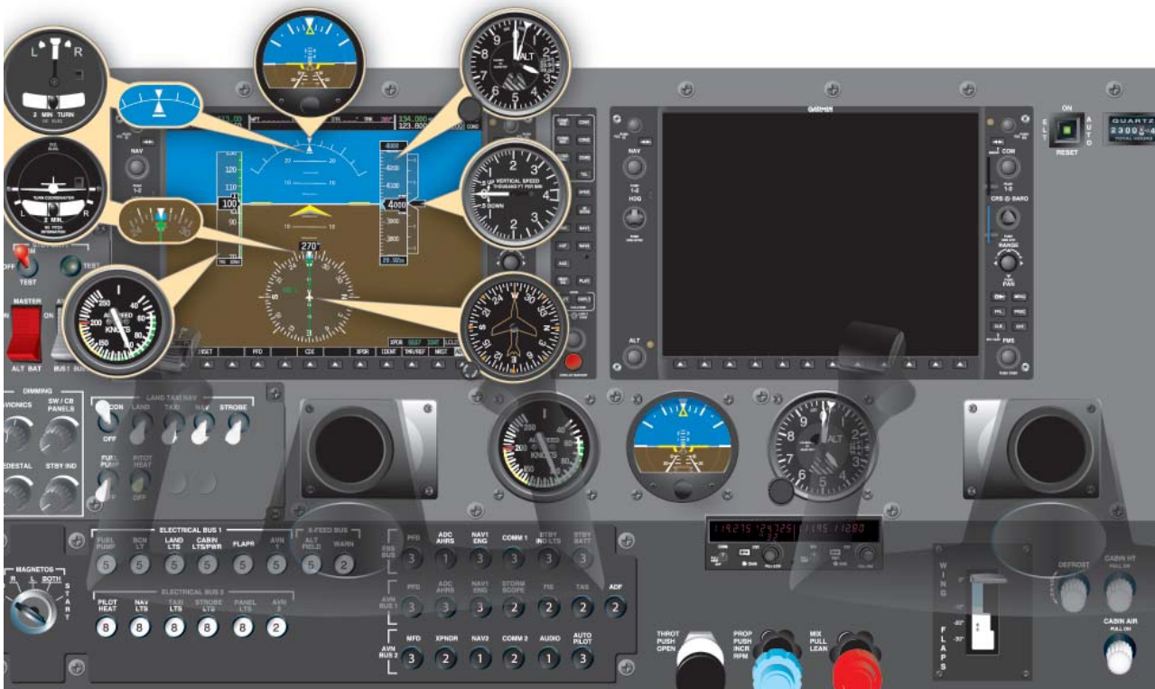
Figure 4-21. Primary Flight Display (PFD) and Analog Counterparts.
