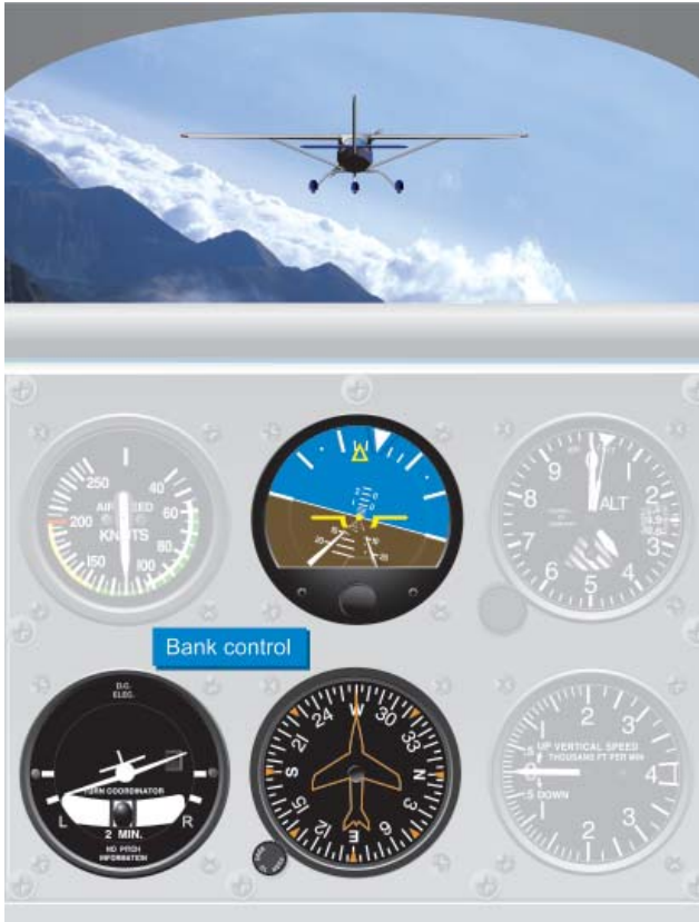
Figure 5-16. Instruments Used for Bank Control.
