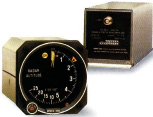
Figure 3-51. Components of a Radar Altimeter.
